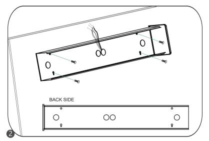
Punch any of the knockouts for power supply wires and make connection. Use (4) screws to install the fixture on surface.
